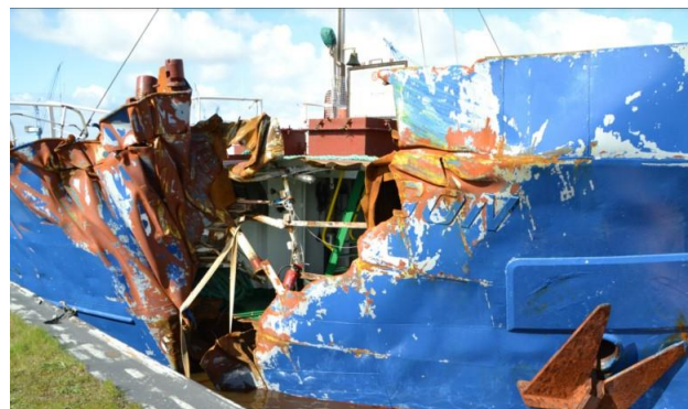
Fig. 1b. The cargo ship Petra L. stroke an offshore wind turbine at Gode Wind 1 wind farm (Germany)
