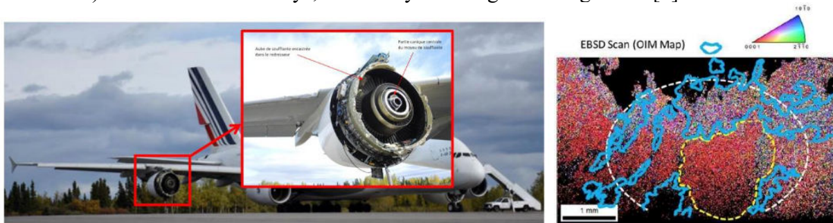
Fig 2: Cold dwell fatigue failure of a motor of an AIRBUS A380-861 exploited by Air France, caused by macrozones [4]
