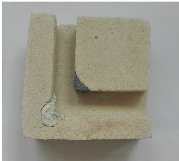
Figure 22 Cutaway of the trimaterial sand mold
